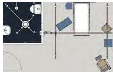
Long Term Care Traverse System with resident access into bathroom with turntable
